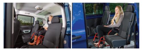
This is the most common type of WAV where the wheelchair user travels as a passenger in the rear of the car either behind the rear passengers (third row) or alongside them (second row). These types of WAV come in all shapes and sizes. If you're going to be sitting in the back, there are a few more things to consider. Will you be able to speak to the driver? Will you be able to see out of the window?
