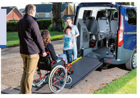
Many WAVs will have had their floor specially lowered to allow enough headroom for the wheelchair user. It also helps make access easier by allowing the ramp to be as short as possible and the angle to be less steep.
