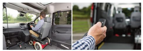
This could be the option for you if you want to drive the vehicle yourself. These WAVs are adapted so that you can operate the driving controls – usually by replacing the pedals with hand controls. It's important to remember you'll need to be able to get in and out of the vehicle yourself. This could involve using a ramp or lift. GM are leaders in drive-from vehicles offering the biggest range of any convertor in the UK. Visit the website for our free Drive-From Wheelchair Buyers Guide.
