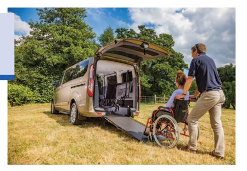
Wheelchair Accessible Vehicles (WAVs) are vehicles that are specially converted so a wheelchair user can travel either as a passenger or a driver.
